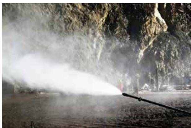
Fig. 5: Fog (water mist) produced from a hand-operated fog gun
